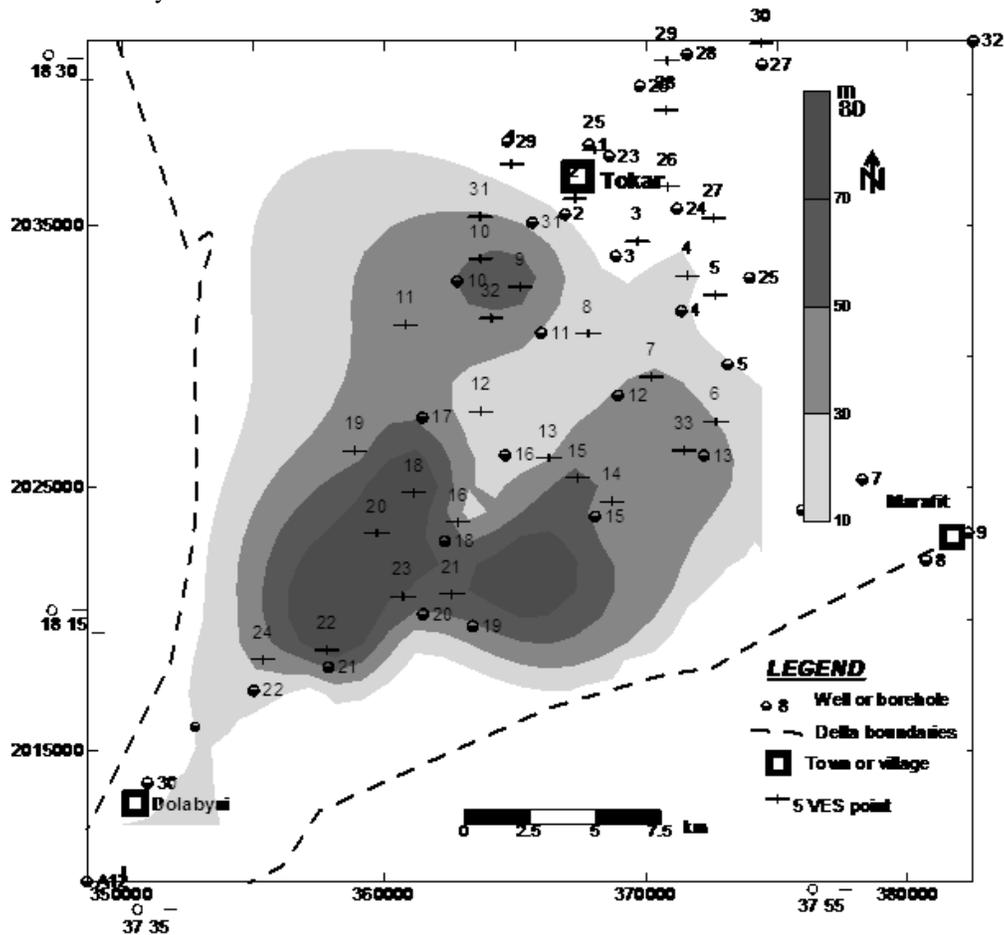
Fig. 3. Freshwater aquifer- thickness map determined by the geoelectric surveys and the borehole data
