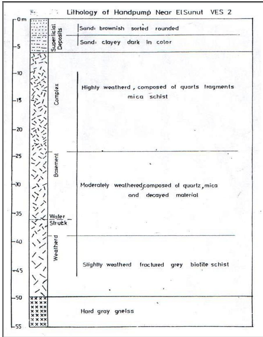
Fig 7: Lithological description of a borehole near VES2
